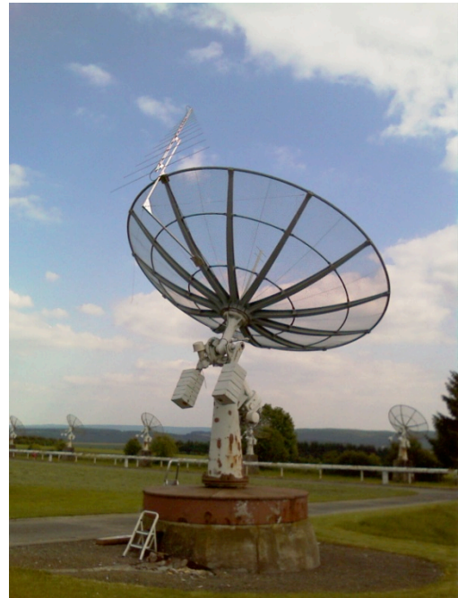
Figure 14: the new 50-1300 MHz log-periodic antenna mounted on the outer ring of a refurbished 6m parabola.
